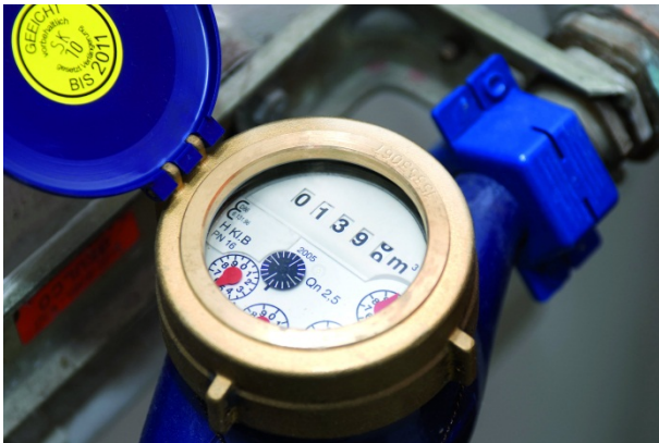
Fig. 1 A conventional vane flow meter for recording the amount of water consumed in a household – today, the measurement of consumption and flow rate is increasingly recorded by ultrasonic sensors
