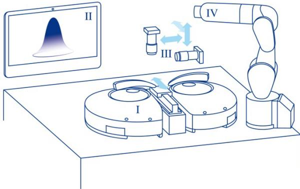
Fig. 3 Schematic design: positioning system for fine adjustment (I), application-specific software and user interface (II), industrial image processing (III) and conventional robotics for pick-and-place of the components (IV) (image: PI)
