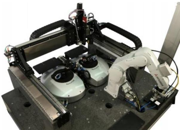
Fig. 1 Automated solution for silicon photonic chip production and inspection: the system integrates several hardware components and software for the automation of assembly and alignment, such as pick-and-place robot technology, image processing, or devices for precision positioning (image: PI)
