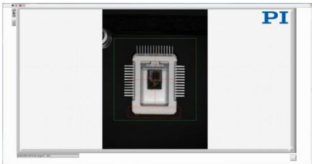
Fig. 4 Integrated image processing supports chip alignment prior to assembly (chip by STMicroelectronics) (image: PI)
