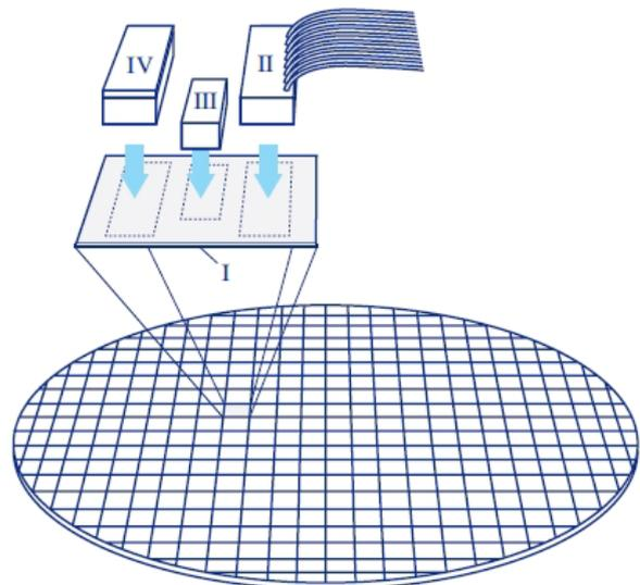
Fig. 2 Chip packaging: silicon substrate (I), fiber connection (II), external laser source (III) and flip-chip bonds (IV) (image: PI)
