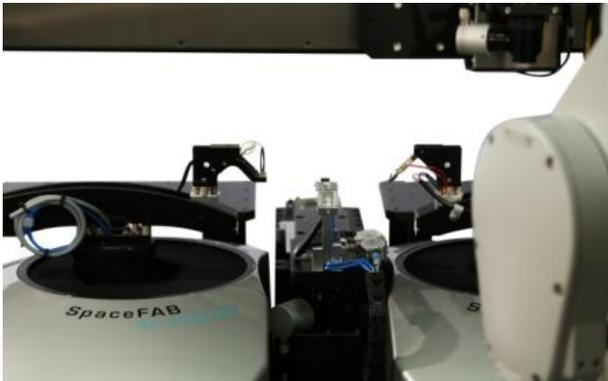
Fig. 6 Exact alignment of the optical fibers on a silicon photonic chip package using two SpaceFab positioning systems (image: PI)
