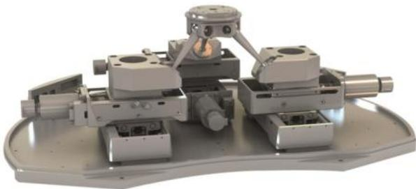
Fig. 7 In contrast to serial kinematics, in parallel-kinematic systems all the actuators act directly on the same platform (image: PI)
