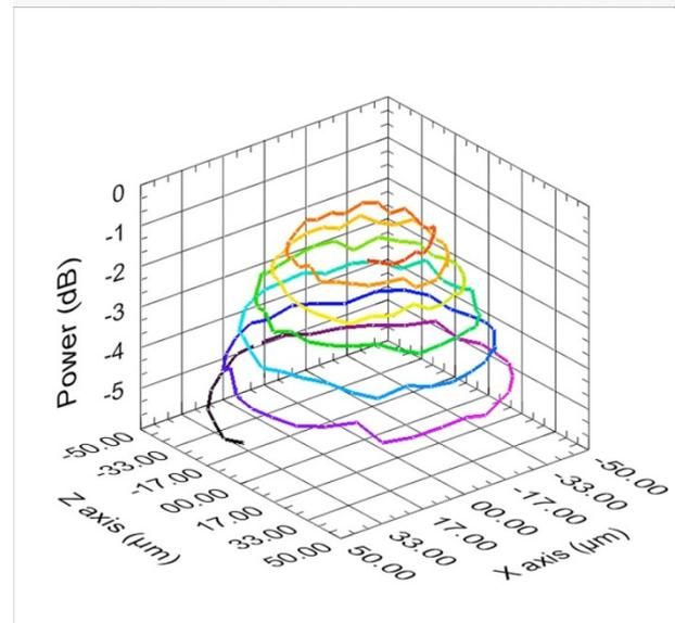
Fig. 5 Fine adjustment for fiber array. The light throughput is measured and optimized via scan algorithms (image: PI)
