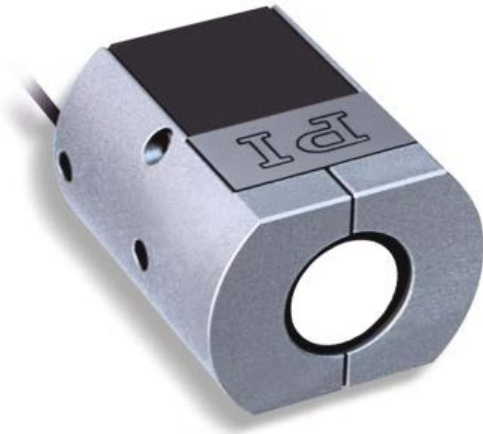
Fig. 5 The piezo-driven tip/tilt platforms are available with tilting angles of up to 3°, which are each offered with position sensors for closed-loop operation or without sensors as fast scanners (Image: PI)
