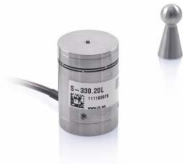
Fig. 1 Highly dynamic, piezo-drive tip/tilt platform with two orthogonal axes and optic deflection angles of up to 20 mrad. Up to four piezo actuators are directly coupled with the moving platform. The length of the actuators determines the tip/tilt angle range; the system is therefore scalable (Image: PI)
