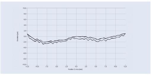
The positioning accuracy of a precision H-824 Hexapod in Z direction over the complete travel range of 25 mm is a few micrometers, and the repeatability is considerably below  $\pm 0.1 \, \mu m$
